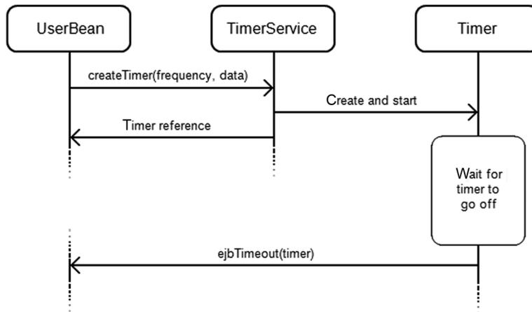
**Figure 13.6** The `TimerService` creating a `Timer` that performs a callback when it times out
