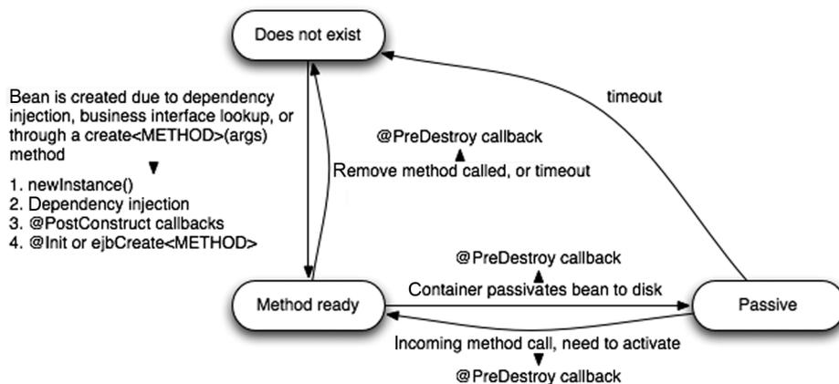
Figure 13.2 Simplified lifecycle of an EJB 3 session bean focusing on the lifecycle callback methods
