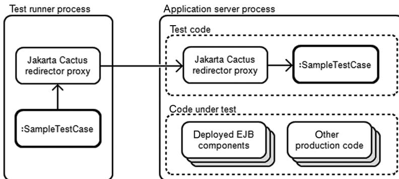
**Figure 13.8** In-container tests using Jakarta Cactus. We run two copies of a `TestCase`. The client-side copy only talks to the server-side redirector proxy, and the server-side copy executes the test logic on request.
