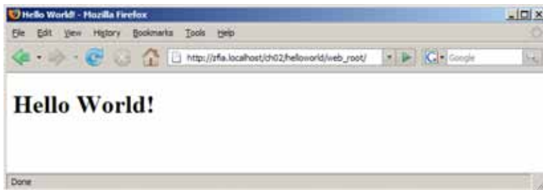
Figure 2.3 The Hello World application produces the words “Hello World!” in our browser. A minimal Zend Framework application requires .htaccess , bootstrap , controller , and view files working together to produce this.
