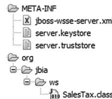
Figure 9.12 Here are the contents of salestax.jar , which contains an EJB-based endpoint, when using WS-Security. The keystore, truststore, and the jboss-wsse-server.xml file are the additional files, as in the previous figure, but the files are placed into the META-INF directory.
