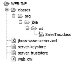
Figure 9.11 Here are the contents of salestax.war when using WS-Security. The additional files, beyond what you saw in figure 9.2, are the keystore, truststore, and jboss-wsse-server.xml file.
