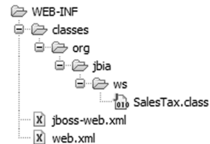
Figure 9.8 Here are the contents of the WAR file for a secured POJO web service. The only additional file, beyond what is listed in figure 9.2, is the jboss-web.xml file.
